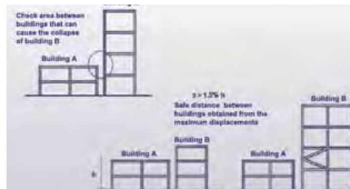
Types of impact between buildings and ways of preventing or avoiding it.
